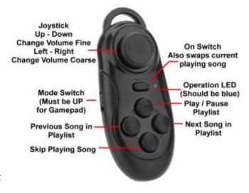
The Mode Switch on the side of the remote must be in the UP position (Gamepad mode) to operate with BallroomDJ. In Ballroom DJ, on the options tab, be sure that "Enable Remote" is checked and that "Bluetooth Gamepad" is selected for the type;
